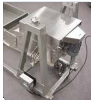
Horizontal motion drive at rear of conveyor is easily accessible and uses a no gear/no oil design.
